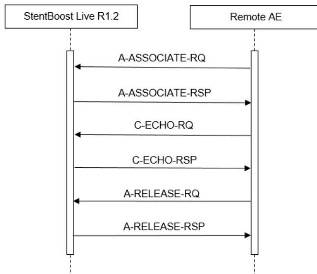
Figure 6: Data Flow Diagram – Verification as SCP
