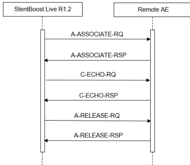
Figure 3: Data Flow Diagram – Verification as SCU
